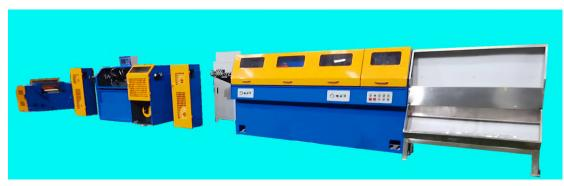
7.Flux cored welding wire forming machine
