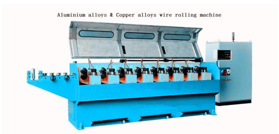
This rolling machine is used for the diameter—reducing processing for alloy materials (such as copper, silver, aluminum, zinc, solder, lead, zinc—aluminum, zinc—solder etc. ) which are difficult to be processed by drawing. Alloy material is able to maintain its plasticity and prevent from cold—work hardening, so as to reducing the processing step of annealing.
